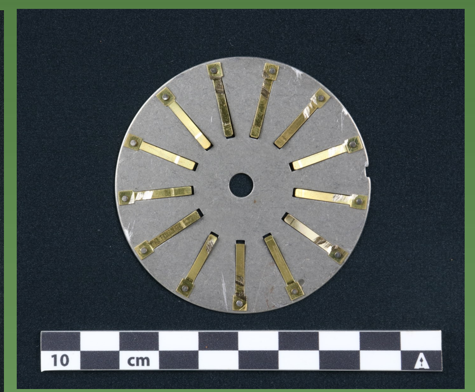
Figure 4: Round reed plate of a modern chromatic pitch pipe.
