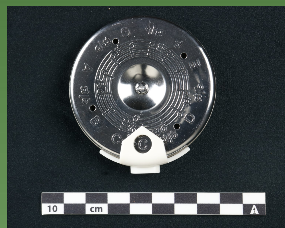
Figure 3: Exterior of a modern chromatic pitch pipe, with notes marked on the case aligning with reeds inside
